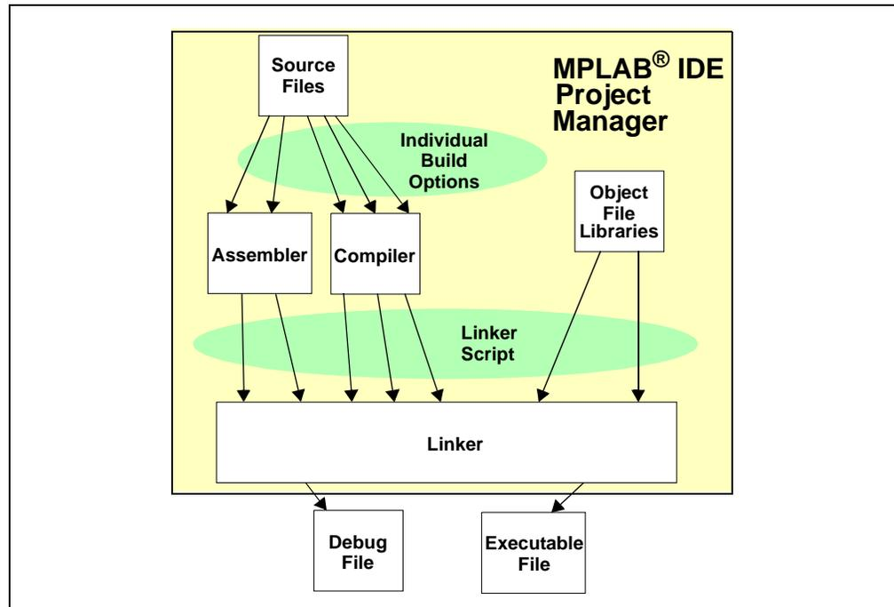
The source files are text files that are written conforming to the rules of the assembler or compiler. The assembler and compiler convert them into intermediate modules of machine code and placeholders for references to functions and data storage. The linker resolves these placeholders and combines all the modules into a file of executable machine code. The linker also produces a debug file which allows MPLAB IDE to relate the executing machine codes back to the source files.
