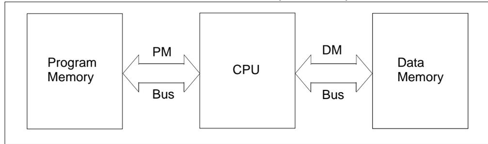
Program memory, or core, instruction length is used to group 8-bit PIC MCUs. Data memory is 8-bit for these devices.
