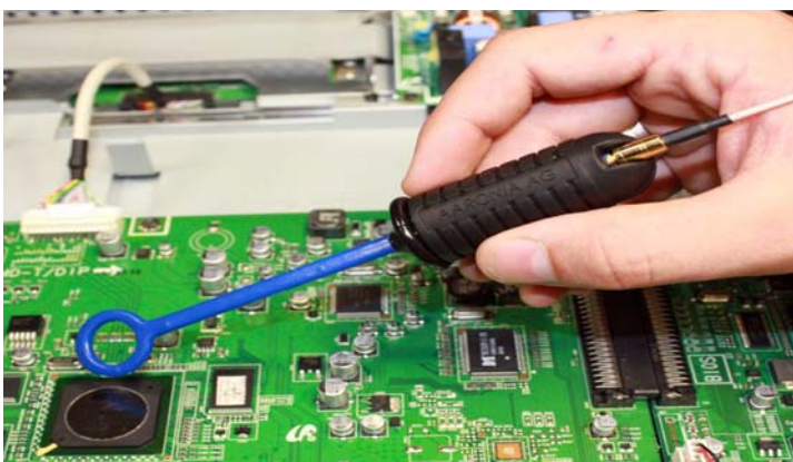
Pinpointing interference sources on a circuit board
