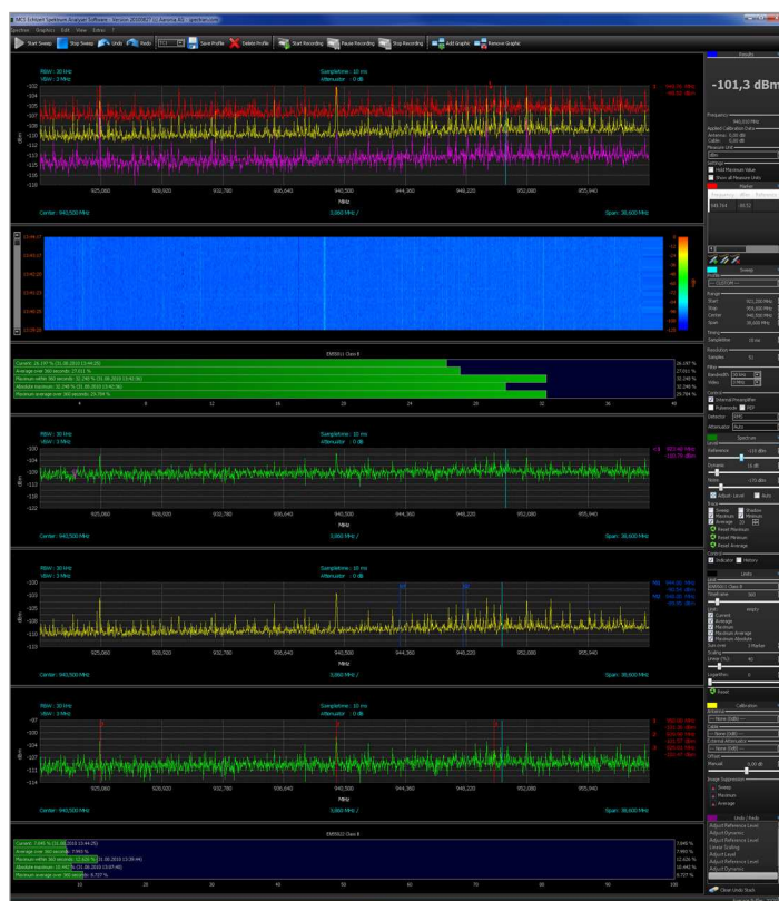
Multi-Window View with Display of multiple views at the same time e.g. Spectrum view (min, max, avg and current sweep), waterfall, limits, histogram, daylog. The MCS Software supports as many windows as wanted (Multi-Window).
