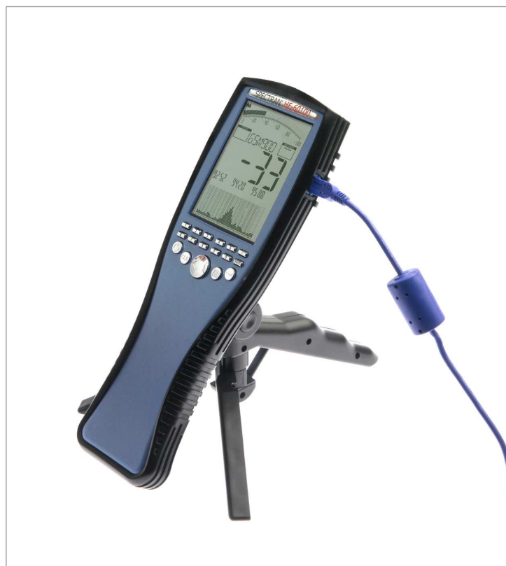
The connection of the SPECTRAN to a PC is realized by the USB-interface, the control is done by the software only (remote control function), the transmission of the measurement results from the SPECTRAN to the PC is made in realtime
